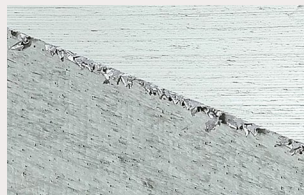
Fine burrs after face milling
