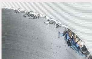
Large burrs after face milling
